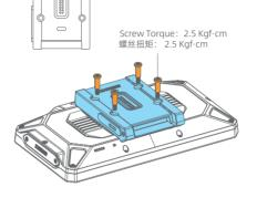
\*The screws are pre-coated with thread locker. \*螺丝已预涂螺纹紧固剂
